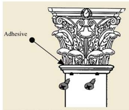
Fig. B – Apply adhesive between the top and bottom of capital.
